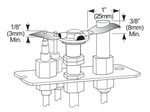
Figure 28. Proper pilot flame appearance.
